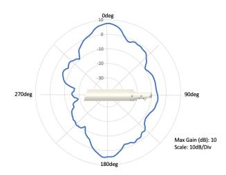
5 GHz Azimuth
