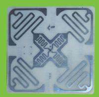
UHF1-Tag7 Omni-directional tag uses Impinj's latest True 3D technology and dual antenna tag. The reading effect is not limited by the reader antenna, can be well recognized anywhere in the space around the card. It is a significant innovative technology in UHF RFID field. Application field include industries including clothes, retail, asset management, and logistics.
