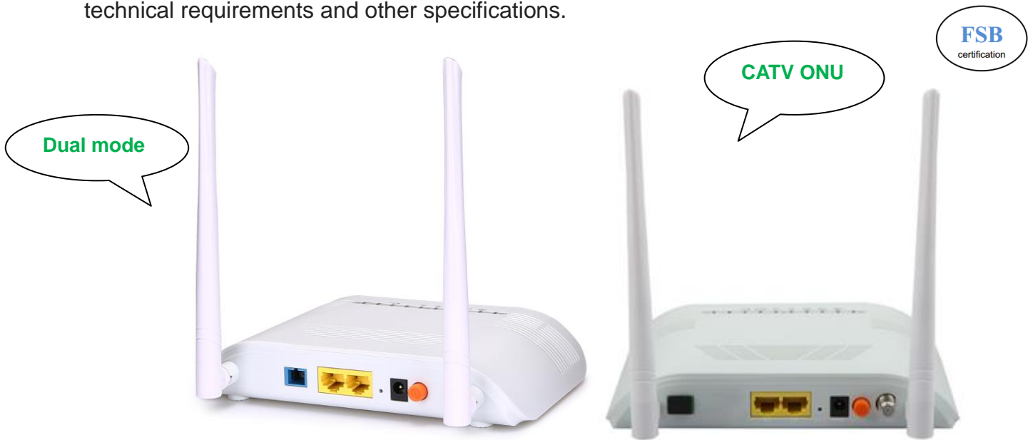
Figure 1 1GE+1FE+WiFi ONU Figure 2 1GE+1FE+WiFi+CATV ONU
