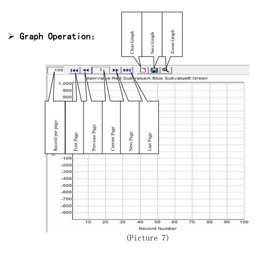
The program records all the data in the measuring process and creates graphs using these data, as shown in picture 7. Within the Graphing Area, functions include: SAVE, CLEAR, GRAPH PAGE SELECTION, and FULL SCREEN. Can also set the range for the data of the graph, size of the graph, and the displaying method. Please see detail below:
