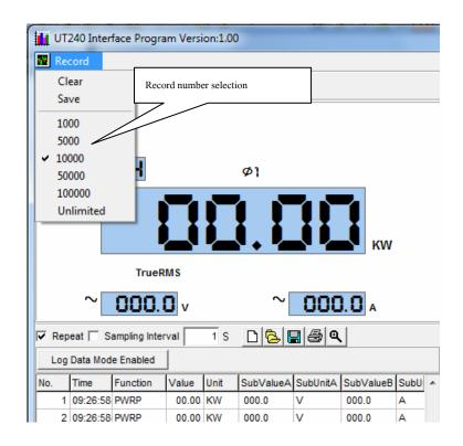
Record Number Selection: Recording stops when total record amount in record area has reached the setting number. For example: the default number is 10000, recording doesn't keep going when the number of record area totals 10000. The software is still running, however does not release any record data and only does it when users change the default. > Control Area( Computer instructions control UT240 corresponding operations )
