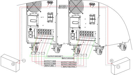
If the UPS is connected to external battery pack, it's required to install battery breaker (DC type) in each UPS. Besides, we strongly suggest to installs a breaker (AC type, D curve) for input/output in each unit. Please refer to UPS user manual for the selection of diameter and color of the wires. **PS.** Each UPS connects to different battery sets.
