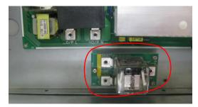
**Step 5:** Connect the OP Relay board to the PSDR board with two short wires, and make the brown wire that removed in step 3 cross the yellow core 5 turns, connect the brown and blue wire to the OP Relay board refer to the following picture, connect the 4 pins brown cable from OP Relay board to PSDR board.
