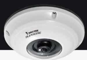
VIVOTEK FE8171V is the first fisheye fixed dome network camera from VIVOTEK, featuring detailed 3.1MP-resolution sensor with superb image quality. Equipped with a fisheye lens for 180° panoramic view (wall mount) or 360° surround view (ceiling/floor/table mount) without blind spots, this camera is able to provide an 8X wider field of view than a standard VGA camera. It is extremely suitable for monitoring open areas such as airports, shopping malls, parking lots, retail stores, offices and more.
